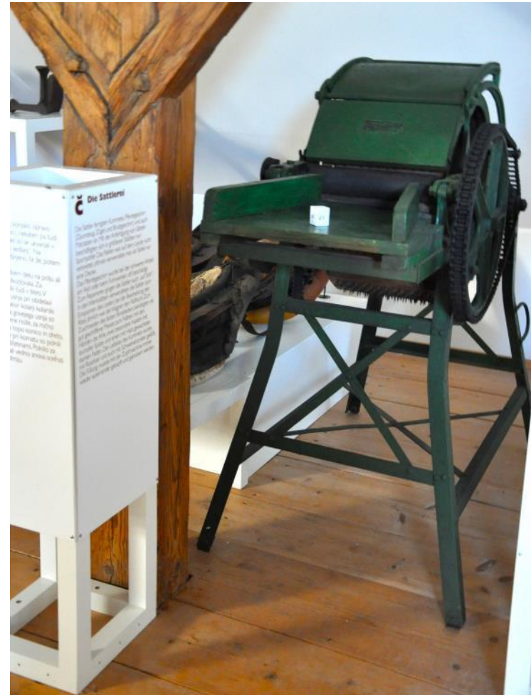
Machine for fluffing and cleaning horsehair, which was used for filling horse collars and mattresses.
